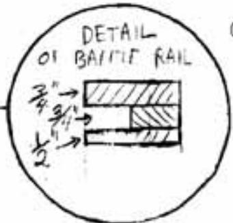
BAFFLE IS 1/2" PLY APPROX. 24X19" CUT TO SLIDING FIT IN RAIL.
